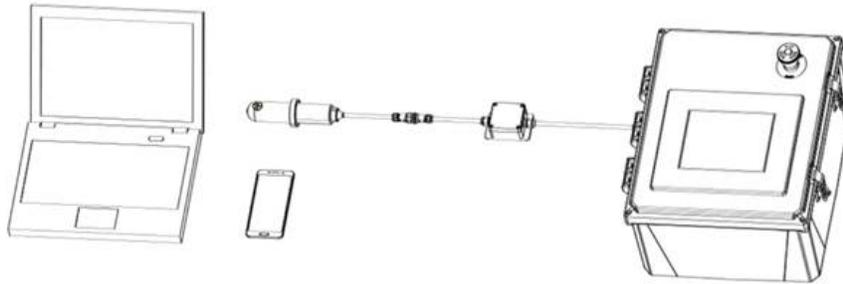
Figure 4. Bluetooth connection to EM-500 sensor
