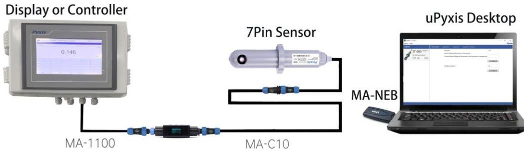
Figure 4. Bluetooth connection to ST-525 Series sensor
