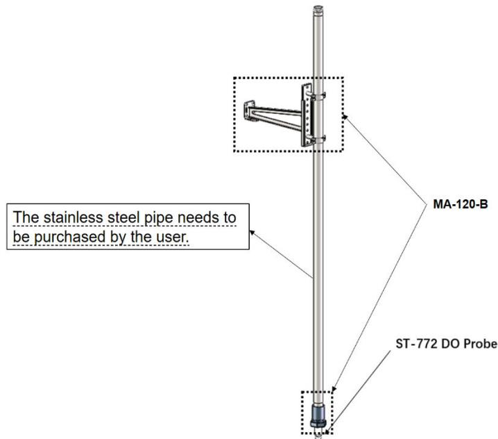
Figure 3 ST-773 in a submersed fixed installation using MA-120-B
